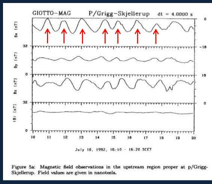
Magnetic field data from Giotto at Comet 27P/Grigg-Skjellerup, nice waves at the water cyclotron period
