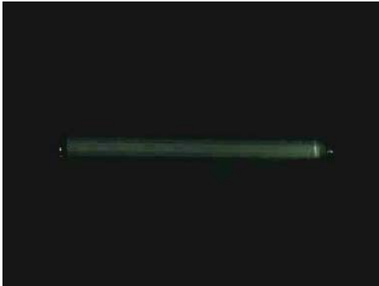
Rubidium-87 vapour cell without buffer gas
